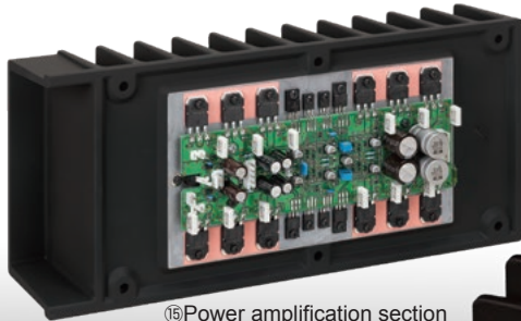
⑮ Power amplification section
